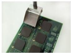
StencilQuik™ allows you to rework a BGA even in tight spaces not accommodated with a metal stencil.
