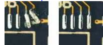
Damaged surface mount pads replaced with new dry film adhesive backed pads.
