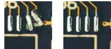
Before After Damaged surface mount pads replaced with new dry film adhesive backed pads.
