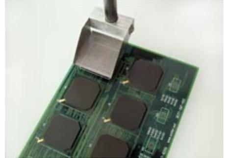
StencilQuik™ allows you to rework a BGA even in tight spaces not accommodated with a metal stencil.
