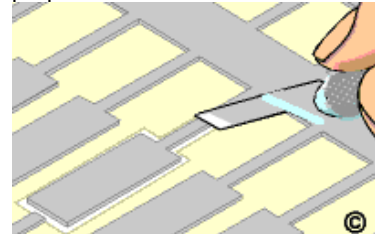
2. Select a replacement pad and trim it out from the Circuit Frame.
